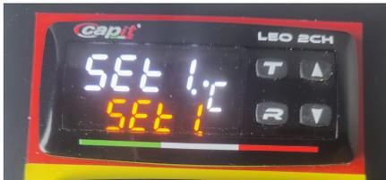
"Leo 2CH" has three pre-programmed set points, both for the "T" tyre and for the "R" rim
