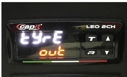
*The sliding Capit text ensures the initial check of all functions, wait 10 seconds before displaying the current temperature (working temperature).*
